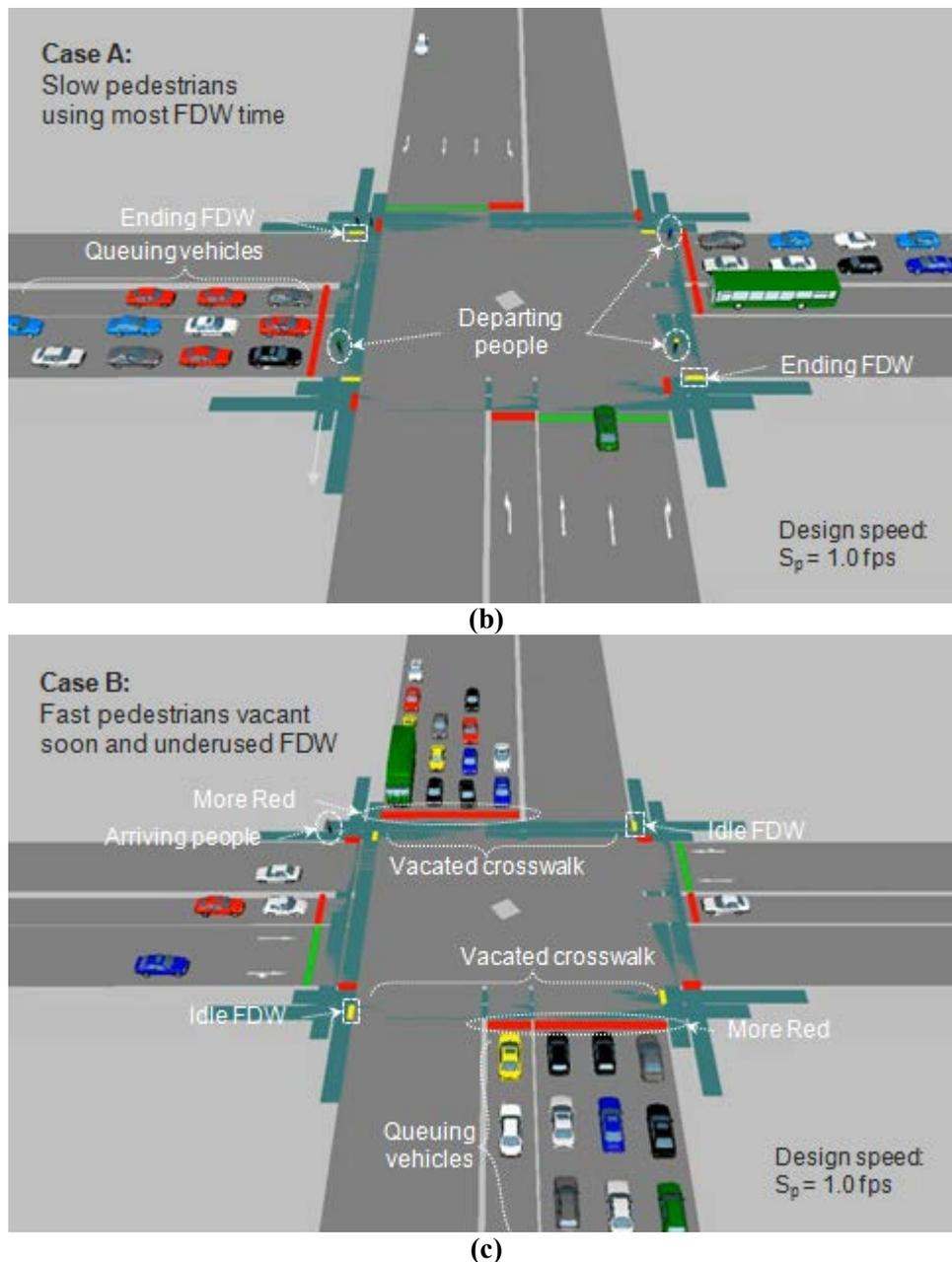
**Figure 1 Problem illustration and simulation animations: (a) “safety versus efficiency” dilemma in signal phase timing, (b) vehicle queuing with slow non-motorized travelers, and (c) vehicle queuing with fast non-motorized travelers.**
