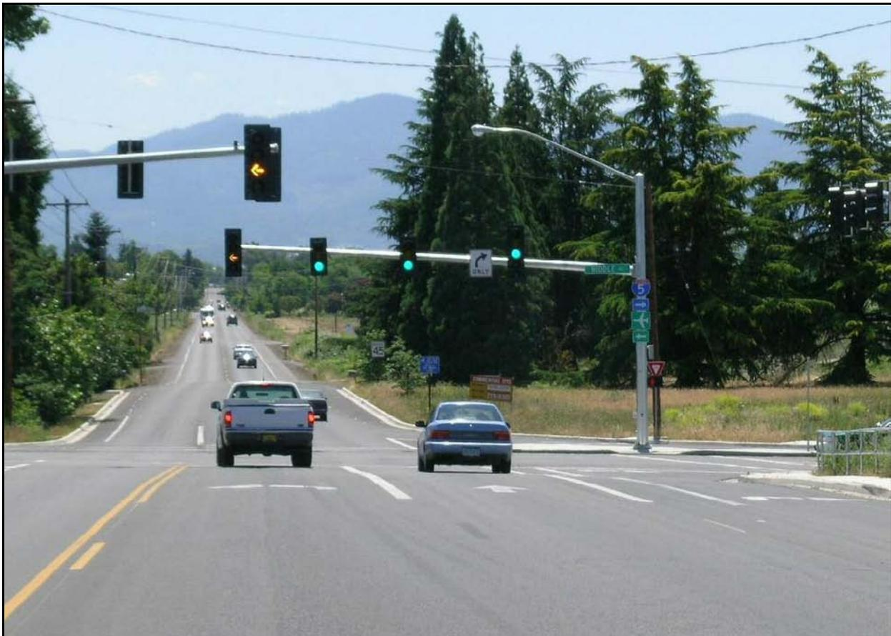
**Figure 1 Field installation of the FYA permissive indication.**
