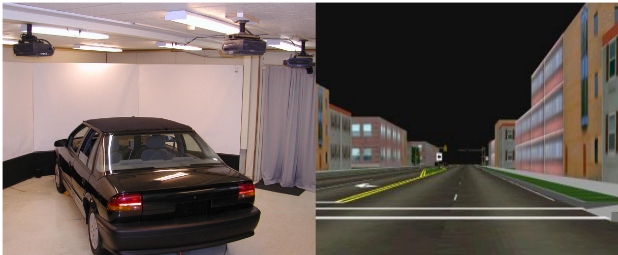
FIGURE 3 Driver simulator vehicle and configuration (left) and sample simulated visual world (right).
