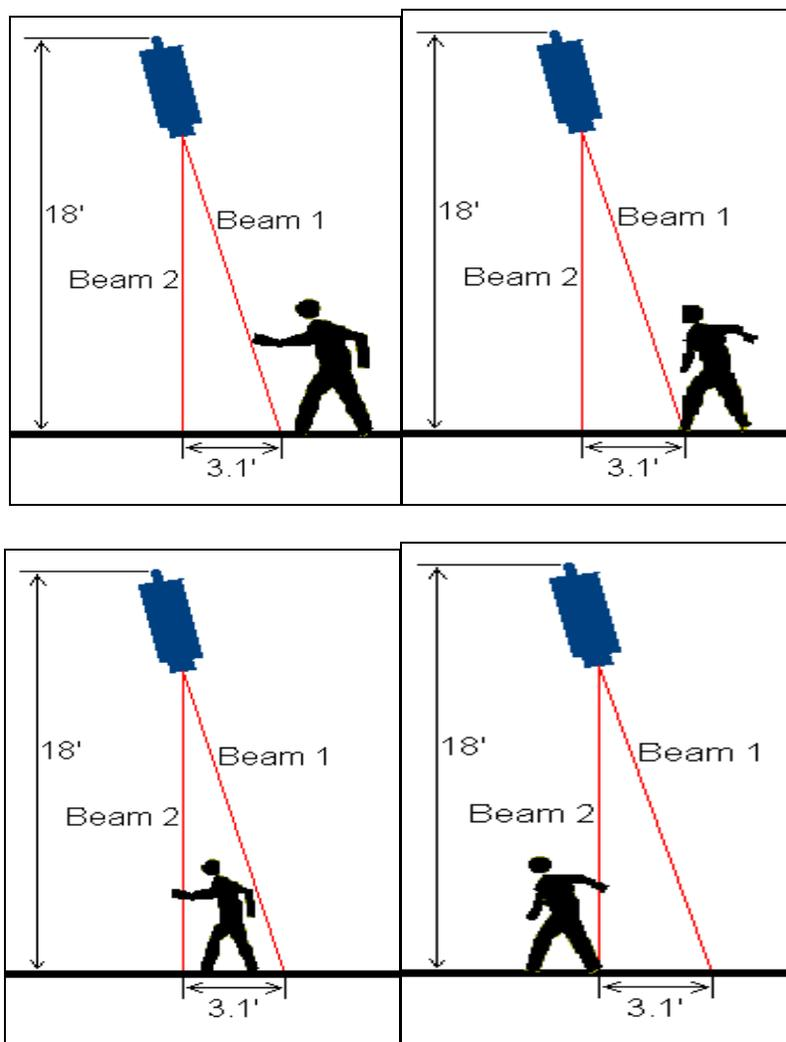
**FIGURE 7 Pedestrian movement underneath the sensor.**
