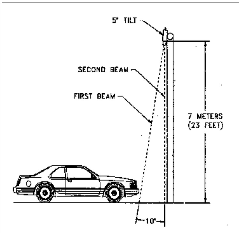
**FIGURE 2** Active-infrared device mounting angle (6).
