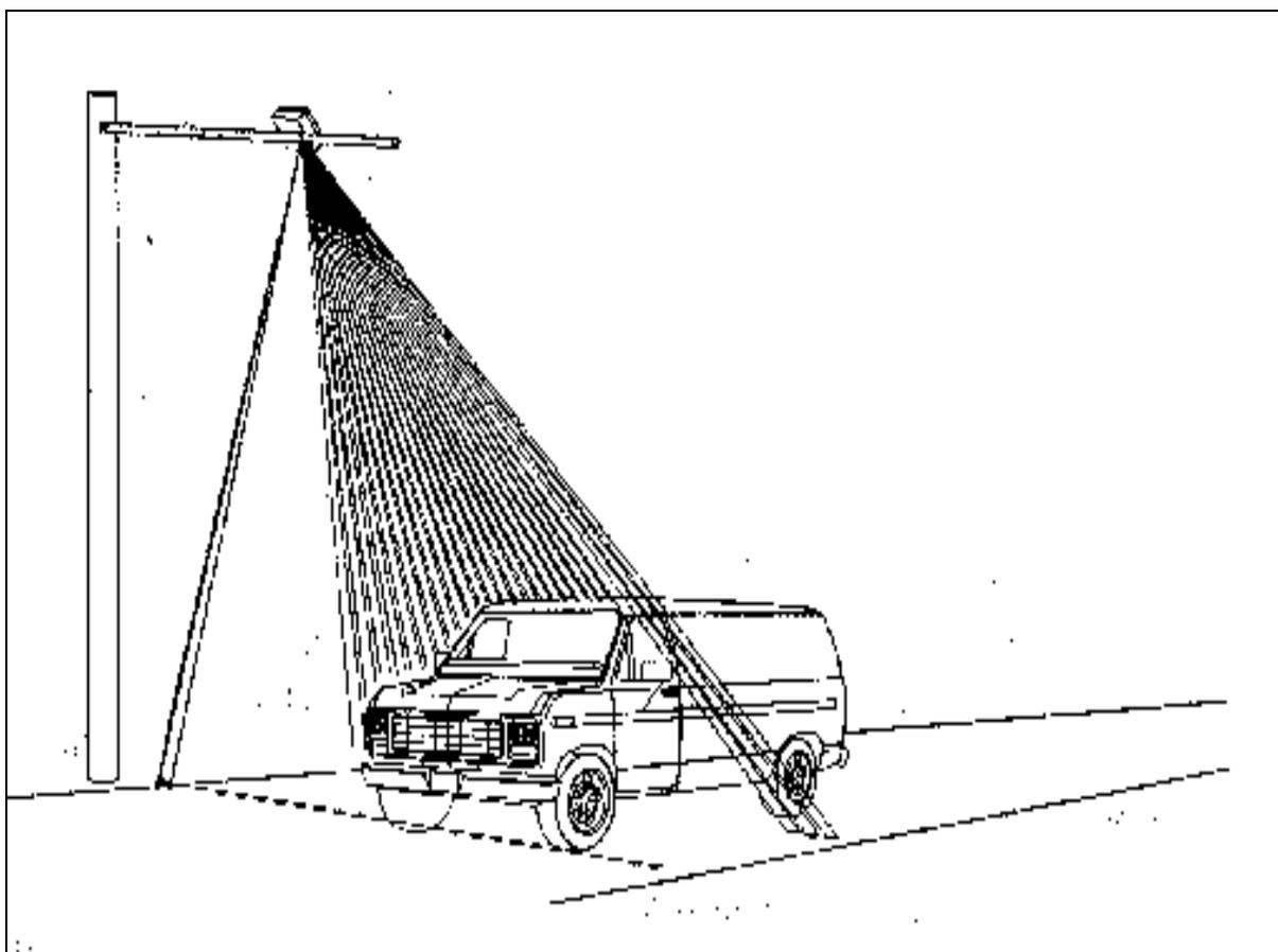
**FIGURE 1 Typical active-infrared scan pattern (6).**
