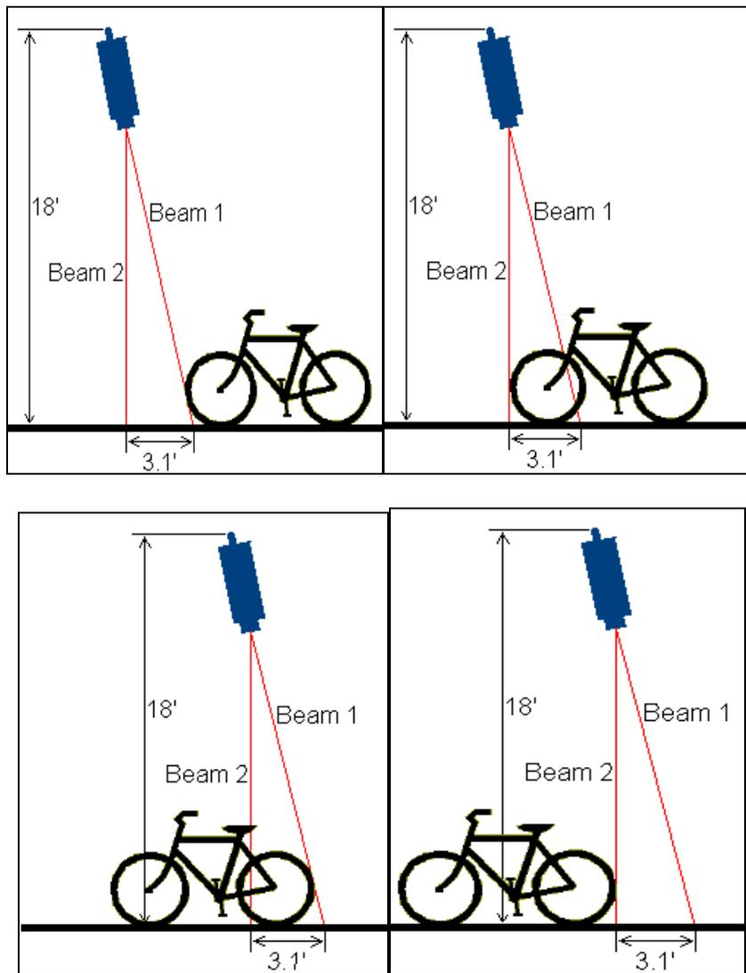
**FIGURE 6 Bicycle movement underneath the sensor.**
