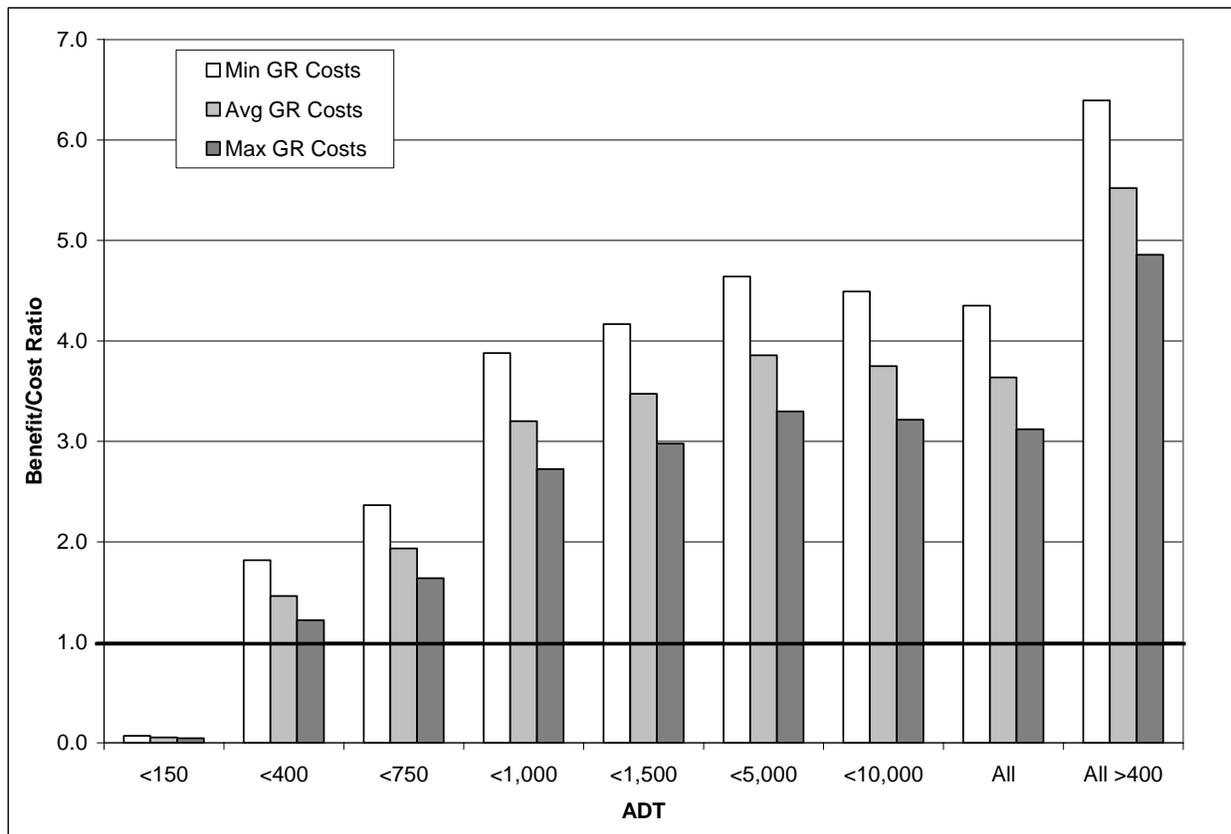
**FIGURE 8 Benefit/Cost ratios for bridge approach guardrail based on cumulative ADT and guardrail installation and maintenance costs.**
