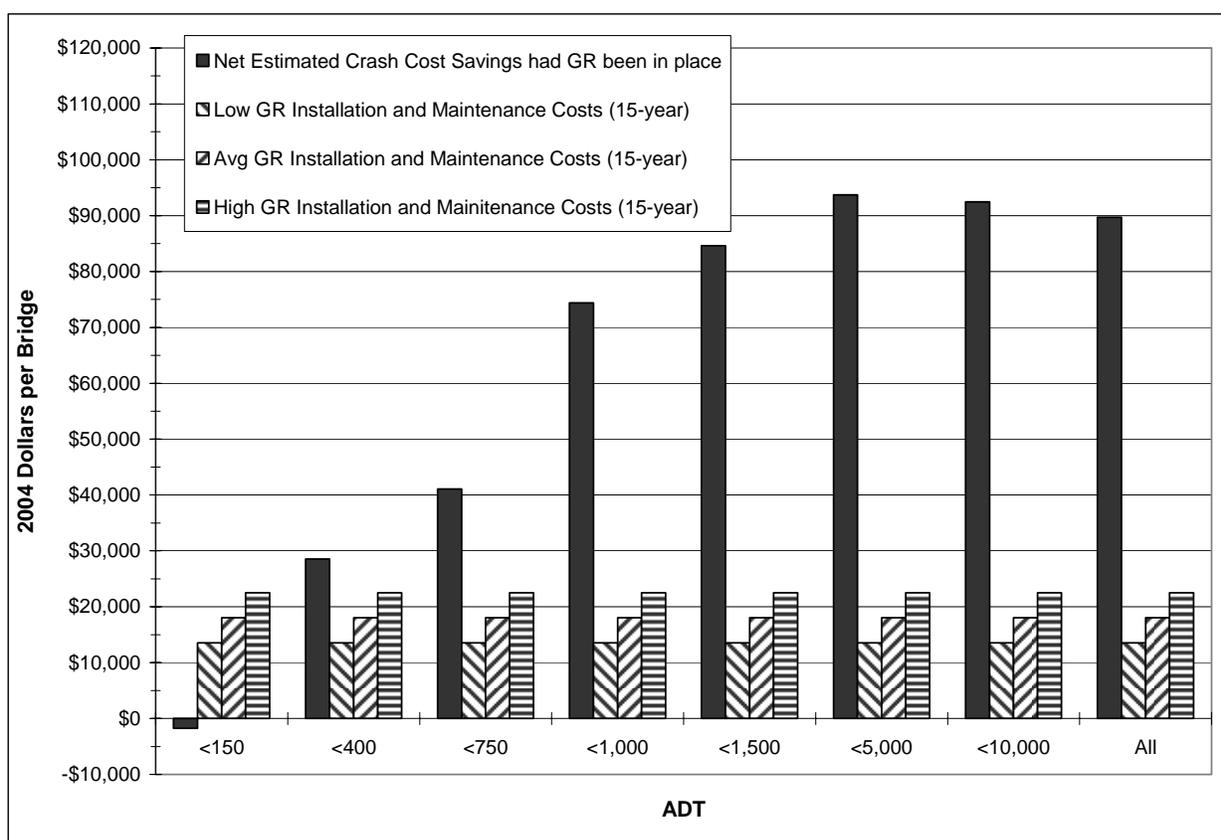
**FIGURE 7 Predicted crash savings and costs per bridge if approach guardrail is installed.**
