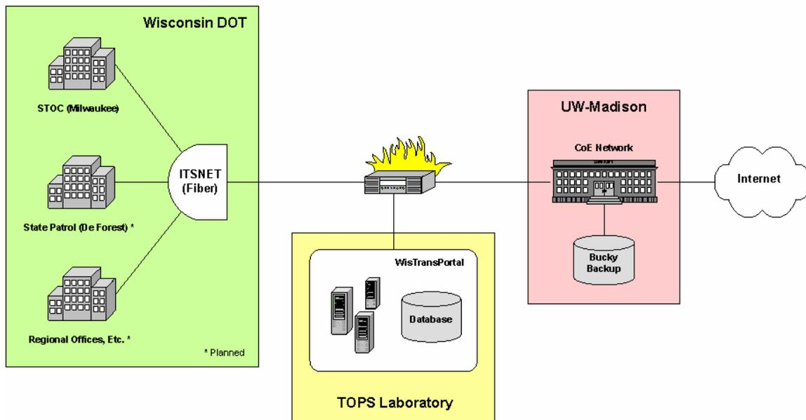
**FIGURE 1** High level overview of the WisTransPortal network architecture. The WisTransPortal sits directly on the UW College of Engineering network and connects to WisDOT over the ITSNET fiber backbone or via the internet.
