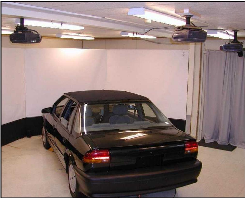
**Figure 4 UMass Human Performance Laboratory driving simulator.**
