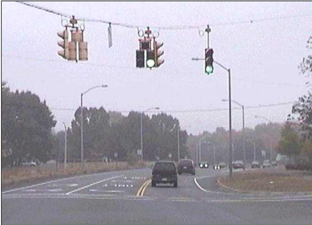
**Figure 1 Example of common PPLT signal display using a shared signal head.**
