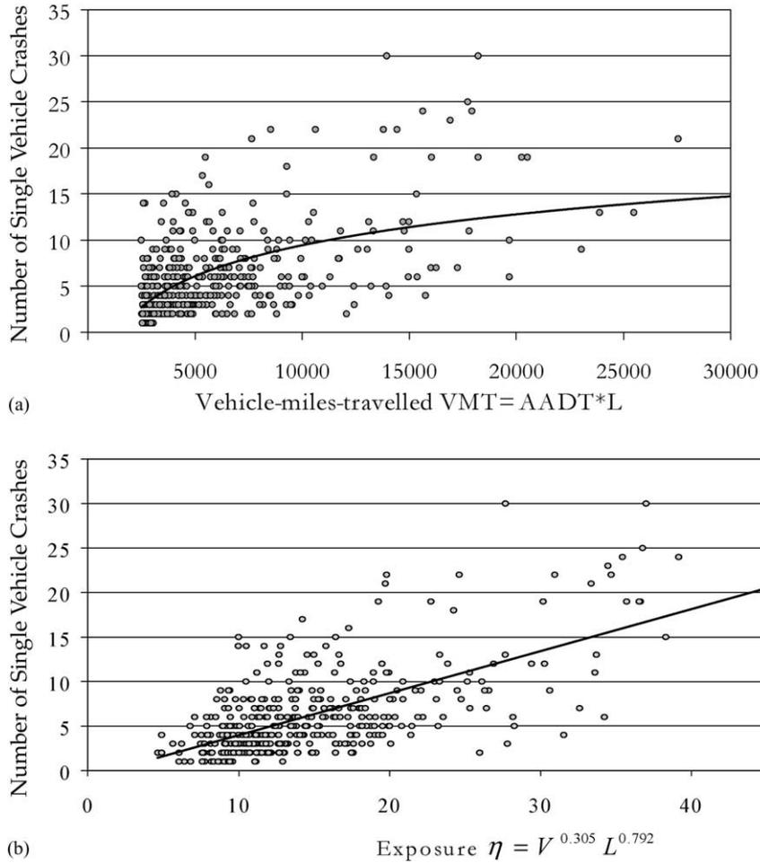
Fig. 4. (a) The observed and predicted crash counts vs. VMT and (b) estimated exposure function for crash type 1.
