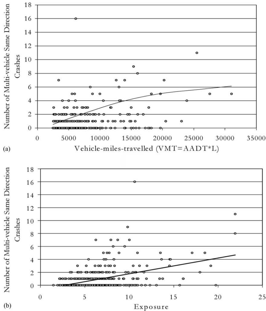
Fig. 5. (a) Observed and predicted crash counts vs. VMT (b) and estimated exposure function for crash type 2.
