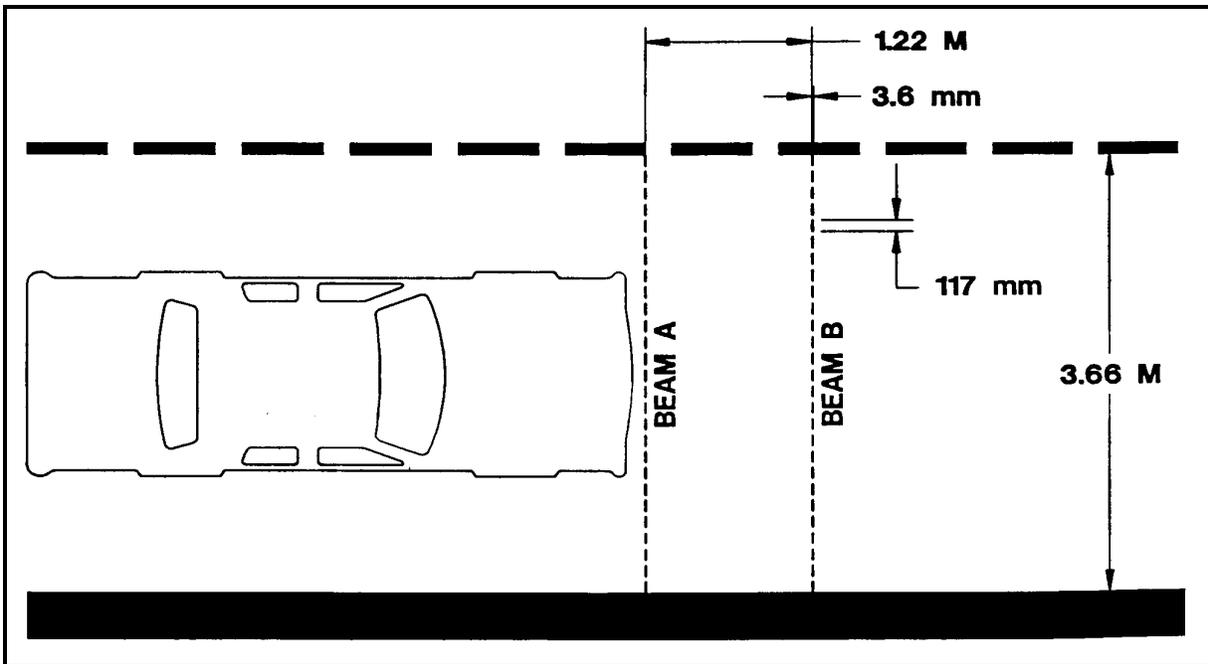
**Figure 5 Plan of the laser beams on road surface (10).**
