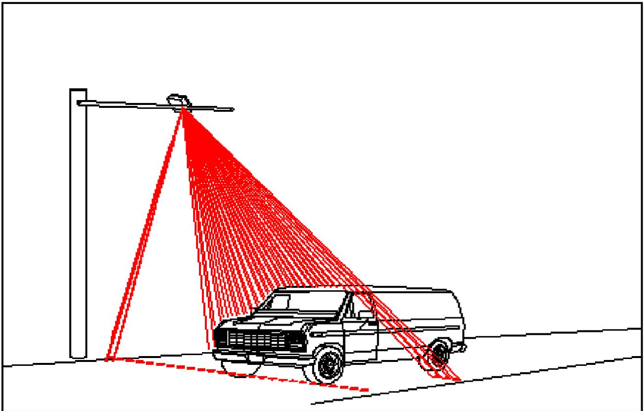
Figure 4 Working of an Active Infrared Detection Device (11).
