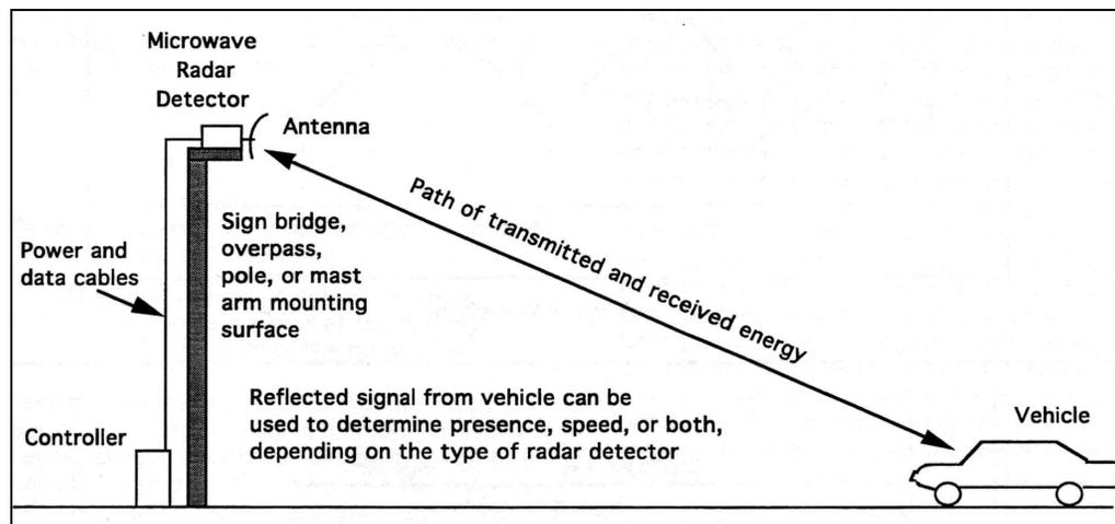
Figure 1 Microwave radar detector (7).
