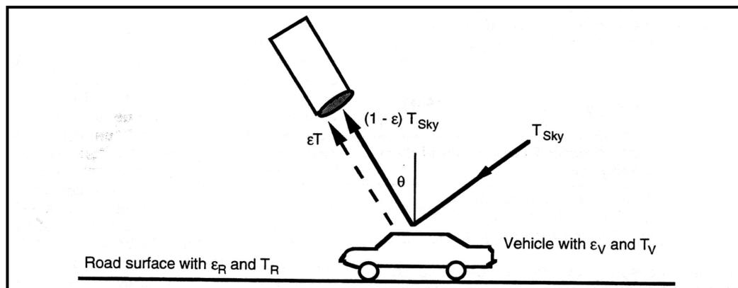
Figure 2 Passive infrared detection (7).
