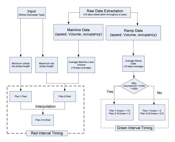
Figure 4 Interval Timing Flow Chart for AM Peak Period
