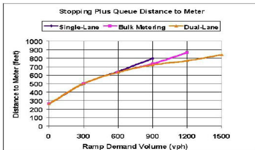
Figure 1-10. Optimum distance from the center of an upstream signalized intersection to a ramp meter for various traffic demand levels 8
